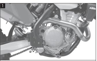
To mount the X-Power, begin by unscrewing the bolt (D) and lowering the rear brake pedal.
