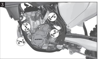
Remove 4 OEM ignition cover bolts exactly as indicated in the image above. Attach the X-Power ignition cover with the remaining 4 (C) bushings and the 3 stock ignition cover bolts and tighten to the OEM torque settings in the owners manual.
