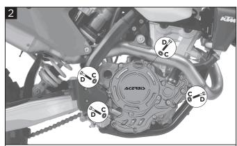
Remove 4 OEM clutch cover bolts exactly as indicated in the image above. Attach the X-Power clutch cover utilizing the 4 OEM bolts and 4 of the included (C) bushings and then tighten to the manufacturers suggested torque settings as indicated in the owners manual. Re-install the rear brake bolt (D) and tighten them to the manufacturers suggested torque settings.
